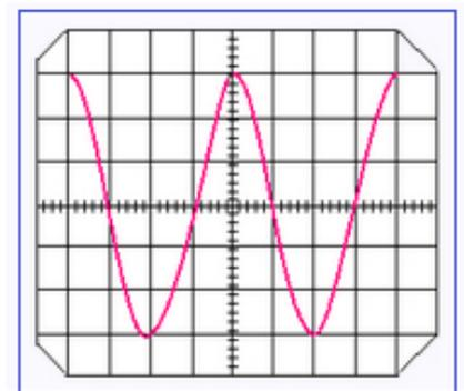
$$U_{max} = y \cdot S_V = 3 \text{ div} \times 2 \text{ V/div} = 6 \text{ V}$$
